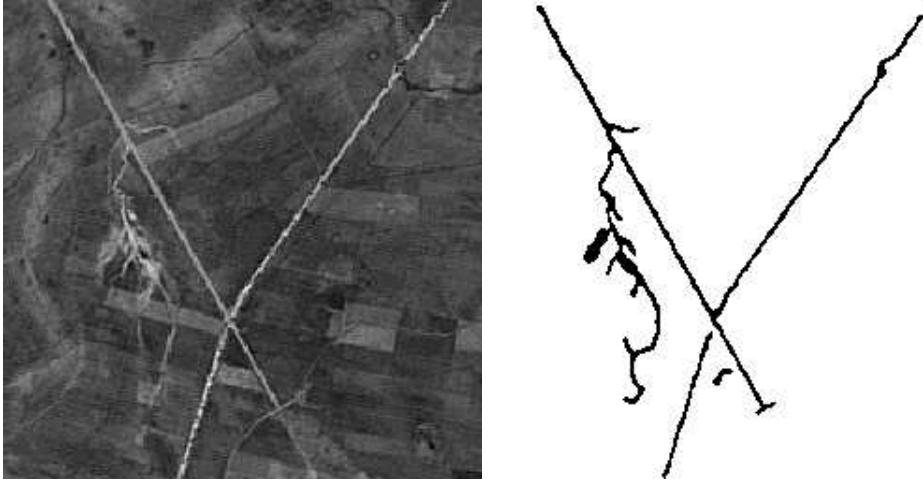
Figure 1: Satellite image (© CNES) and result of line network extraction. Parameter values: [\lambda = 1, \alpha = -0.2, \beta = 0.2, \lambda_i = 2.4, \alpha_i = 0, \beta_i = 2.4] .
