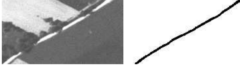
Figure 18: An aerial image (© IGN) with occlusions and the result of applying E = E_0 + E_{\text{gap}} to this image. Parameter values: [\lambda = 1, \alpha = -0.14, \beta = 0.06, \lambda_i = 2.9, \alpha_i = 0.3, \beta_i = 2.9, \beta_A = 6] .
