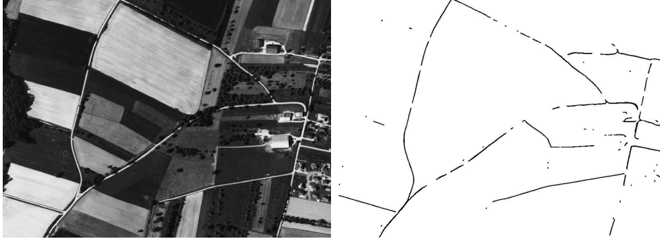
Figure 2: Aerial image (© IGN) and result of line network extraction. Parameter values: [\lambda = 1, \alpha = -0.17, \beta = 0.2, \lambda_i = 2, \alpha_i = 1, \beta_i = 2] .
