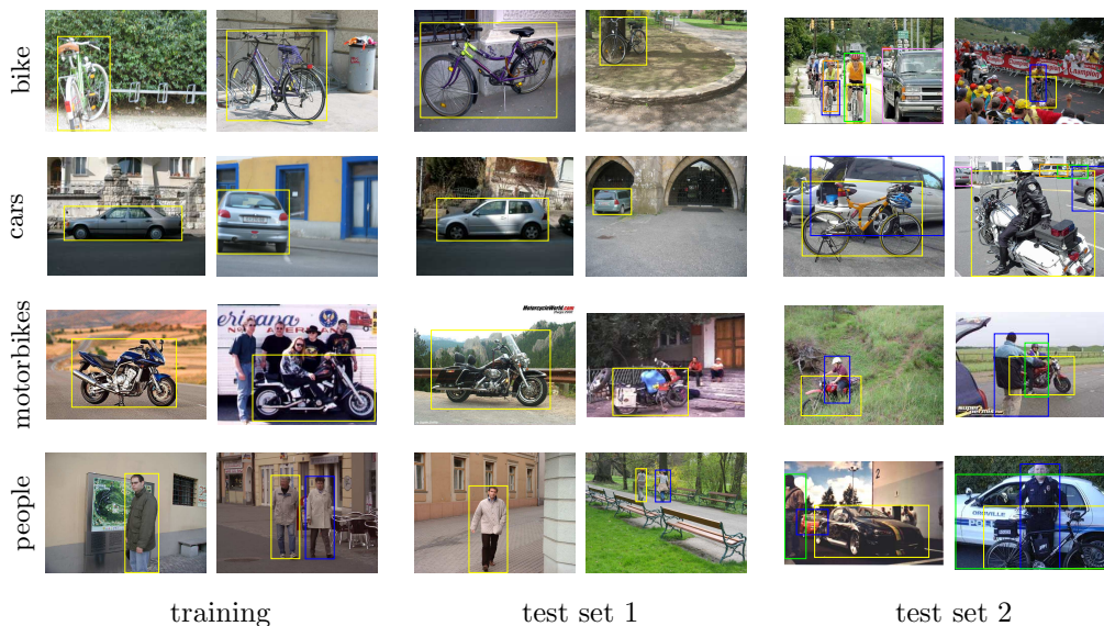
Figure 9: Image examples with ground truth object annotation of different categories of the PASCAL challenge. The dataset may be obtained from http://www.pascal-network.org/challenges/VOC/voc/index.html .
