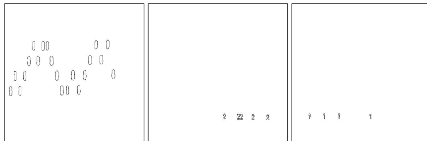
Figure 8.11: Grouping with respect to orientation, elongation, diameter, and a convexity coefficient. The DNA marks are the most meaningful group NFA_g = 10^{-10} . It is worth noting that the 1 and 2's, though not meaningful groups, have NFA_g only slightly larger than 1 (1.6 and 4.5).
