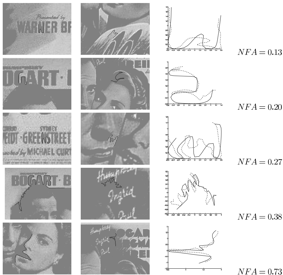
Figure 7.17: The five false matches for NFA < 1 , with their normalized shape elements. The left most and middle images correspond to the query and the scene shape elements, respectively. The right most image shows their normalized shape elements, superimposed. All false matches show NFAs between 0.1 and 1
