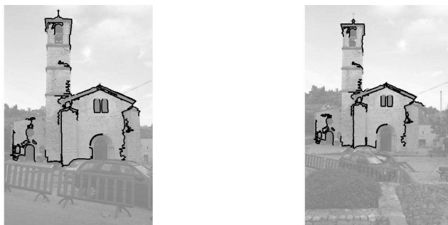
Figure 10.10: Église de Valbonne: a single maximal meaningful group is detected. All false matches and spatially incoherent matches are rejected. The group contains 35 (similarity invariant) meaningful matches and -\log_{10}(NFA_g) = 84.8 .
