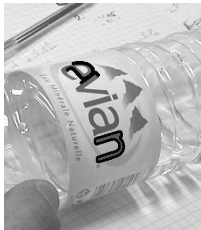
Figure 7.33: Evian: global similarity invariant matching. All 1-meaningful matches with character ‘n’ from the query image. The query ‘n’ is represented with 10 global shape elements, that match with 36 global shape elements from the scene image. The lowest NFA is 10^{-11} . False detections show NFAs between 0.7 and 1
