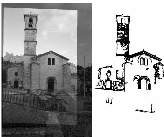
Figure 10.11: Église de Valbonne: registration of the images computed from the maximal meaningful group. On the right, the matching pieces of level lines. On the bottom right image, some straight lines appear, because of the coincidental superposition of the lower and upper part of the gate after registration.
