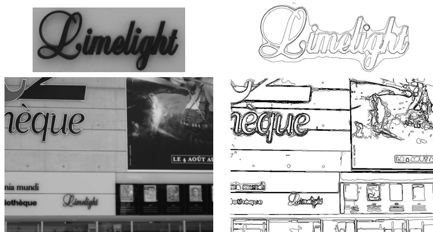
Figure 7.22: Top row: Query image and its maximal meaningful boundaries; 312 shape elements were extracted from this image. Bottom row: Scene image and corresponding maximal meaningful boundaries. 1,859 shape elements were extracted from it
