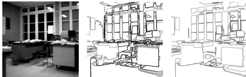
Figure A.4: Regularity detectability. The original is the left most. In middle, the 204 detected contrasted smooth boundaries as defined in Def. A.2. On the right, the 96 smooth boundaries, with no contrast information, defined in (A.8). All the main boundaries are already present. Of course, contrast may be the main cause of small NFA, since regularity acts at larger scales. For instance, the window panes have NFA about 10^{-150} with contrast and 10^{-15} with regularity only (which still make them detectable in an image database containing 10^{15} images, which is far larger than any existing database). The desk on the bottom right has a NFA equal to 10^{-60} with contrast and 10^{-20} with regularity, which is already very small
