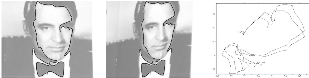
Figure 7.11: Similarity invariant semi-local recognition method: The match showing the lowest NFA ( 3.8 \cdot 10^{-8} )
