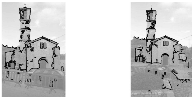
Figure 10.9: Église de Valbonne: 81 meaningful matches were found, for 14,710 shape elements in the target image and 18,413 in the scene image. All false detections have NFA larger than 0.1. The best match has NFA = 2.98 \cdot 10^{-12} .
