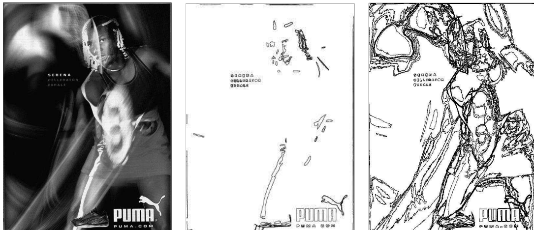
Figure 3.6: Influence of quantization noise on meaningful boundaries. On the left, the original image is coarsely quantized since it has a very low contrast. This leads to bad gradient estimation and a lot of missing detections (middle). Multiscale detection is less sensitive to quantization noise and leads to more correct detections (right)
