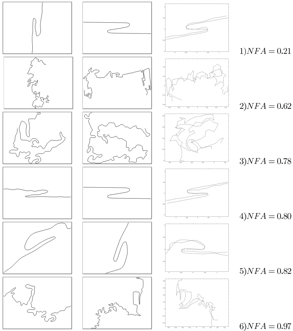
Figure 7.19: The six false matches detected for NFA < 1 , with their normalized shape elements. The left most and middle images correspond to the query and the scene shape elements, respectively. The right most image shows their normalized shape elements, superimposed. All false matches show NFAs between 0.1 and 1
