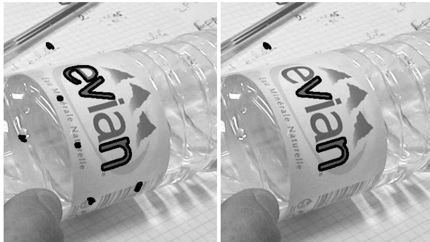
Figure 7.34: Evian: affine invariant global matching. Meaningful matches with character ‘n’ from the query image, represented with 10 global shape elements. Left: 1-meaningful matches, 35 matches. False matches show an NFA between 10^{-3} and 1, but some of them are not really “false” but “casual” matches, since they correspond to other characters ‘n’ and ‘u’ which are present in the scene. Good matches show NFA ranging from 10^{-15} to 10^{-8} . Right image: the 23 meaningful matches showing NFAs below 10^{-2}
