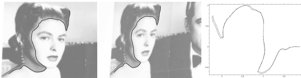
Figure 7.9: Affine invariant semi-local recognition method: The match showing the lowest NFA ( 6.5 \cdot 10^{-11} )
