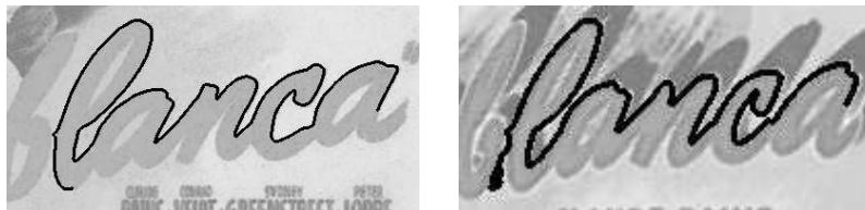
Figure 7.16: The match with the lowest NFA. The query shape element (left image) matches the database shape (right image). NFA = 1.1 \cdot 10^{-6}
