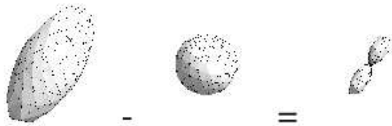
Figure 8: Minimum Inscribed Sphere (MIS) subtraction [21].
