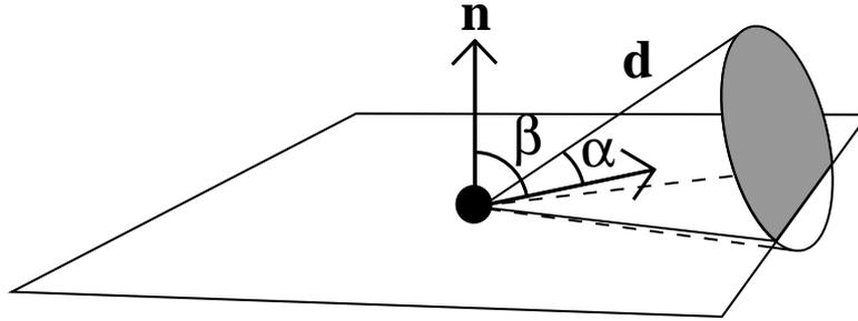
Figure 6: The cone of occluded directions is clipped by the tangent plane to the receiver to give the ambient occlusion value.
