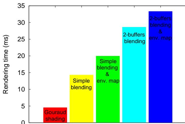
Figure 16: Observed rendering times on our system, depending on the features activated and on the blending method.
