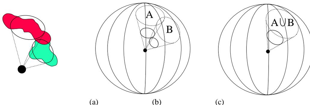
Figure 10: The occlusion from two separate shadow casters (a) are combined by replacing their two cones (b) by a resulting new cone, representing the occlusion of their union (c).
