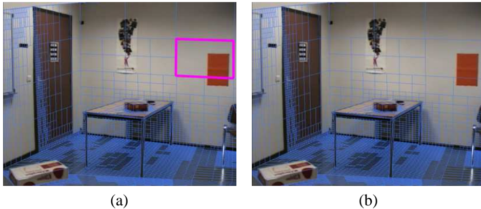
Figure 11: (a) A patch in pink with a different colour than neighbours but the same visibility. The patch was not subdivided. (b) Mesh after texture-based refinement with improved shadow boundaries. Compare to Figure 10.
