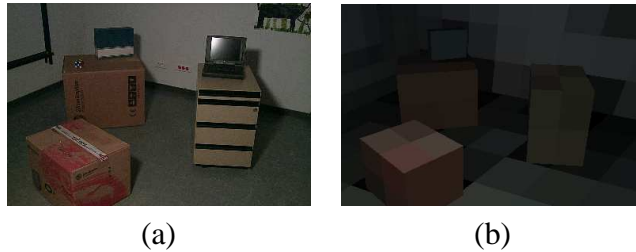
Figure 5: (a) The original view of the scene and (b) the corresponding radiosity mesh used to simulate indirect light and dynamic updates; note the coarse subdivision.
