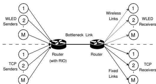
Figure 7: Topology used for testing TCP friendliness.
