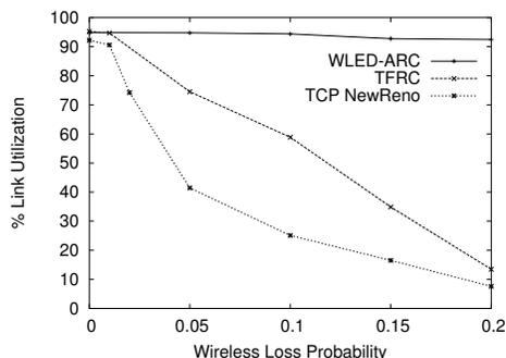
Figure 6: Link Utilization for Different Wireless Loss Probabilities.
