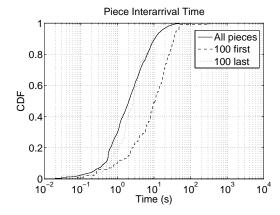
Fig. 7. CDF of the piece interarrival time for torrent 10. **Legend:** The solid line represents the CDF for all pieces, the dashed line represents the CDF for the 100 first downloaded pieces, and the dotted line represents the CDF for the 100 last downloaded pieces.
