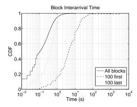
Fig. 8. CDF of the block interarrival time for torrent 10. **Legend:** The solid line represents the CDF for all blocks, the dashed line represents the CDF for the 100 first downloaded blocks, and the dotted line represents the CDF for the 100 last downloaded blocks.
