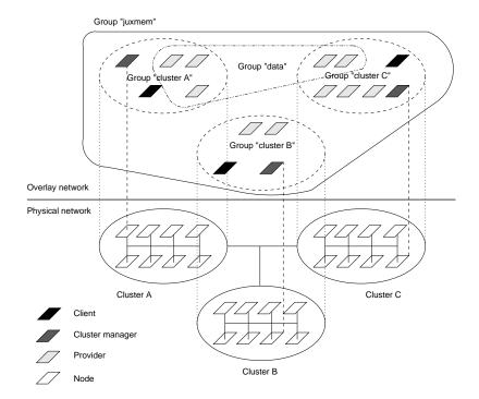
Figure 2. Hierarchy of the entities in the network overlay defined by JUXMEM.
