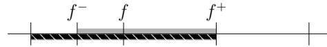
Figure 3: Ulp and faithful rounding when f is a positive power of the radix
