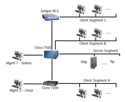
Figure 8-1: PSNC management testbed
