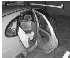
Fig. 1. Side camera system.
