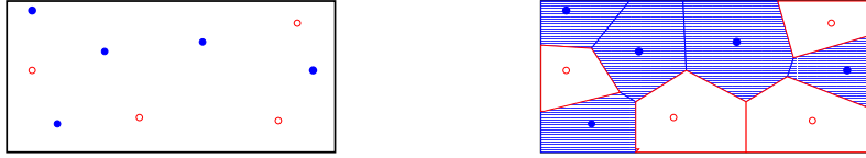
(a) The genotype: a list of labeled Voronoi sites. Black dots are sites with label 0 and white dots are sites with label 1. (b) The phenotype: the Voronoi cells receive the label of the corresponding site, and build a partition of the design domain.
