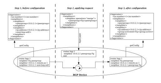
Figure 2: BGP Configuration Constraints
