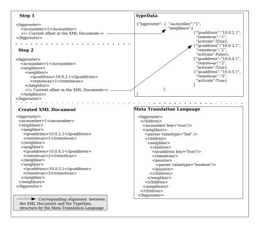
Figure 10: CLI to XML process construction
