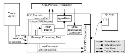
Figure 3: BGP Module's Functional Architecture
