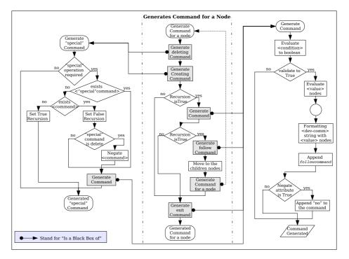
Figure 8: Command Generation process for a node
