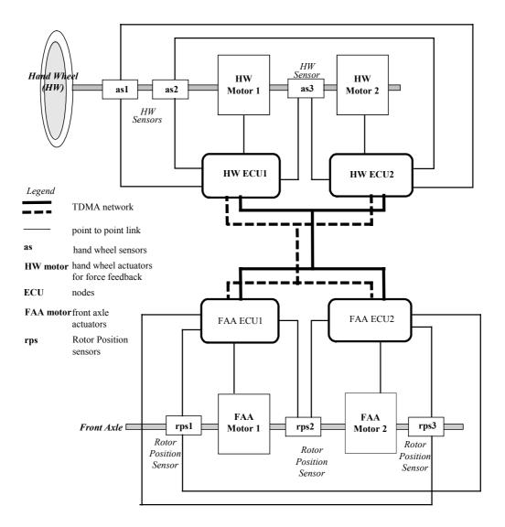
Figure 4: Steer-by-Wire operational architecture
