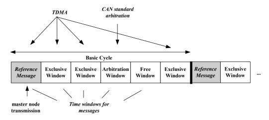
Figure 3: Example of a TTCAN Basic Cycle
