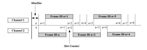
Figure 2: Example of message scheduling in the dynamic segment of the FlexRay communication cycle
