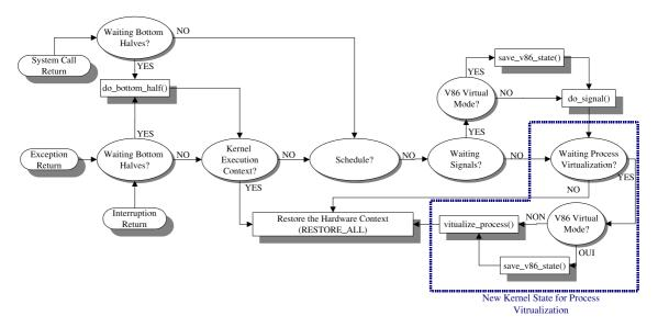
Figure 1: Kernel state for process virtualization
