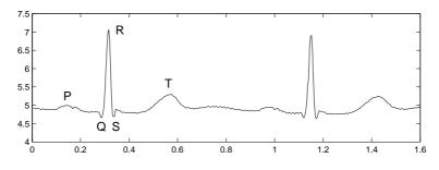
Figure 1: ECG signal and P-Q-R-S-T wave forms
