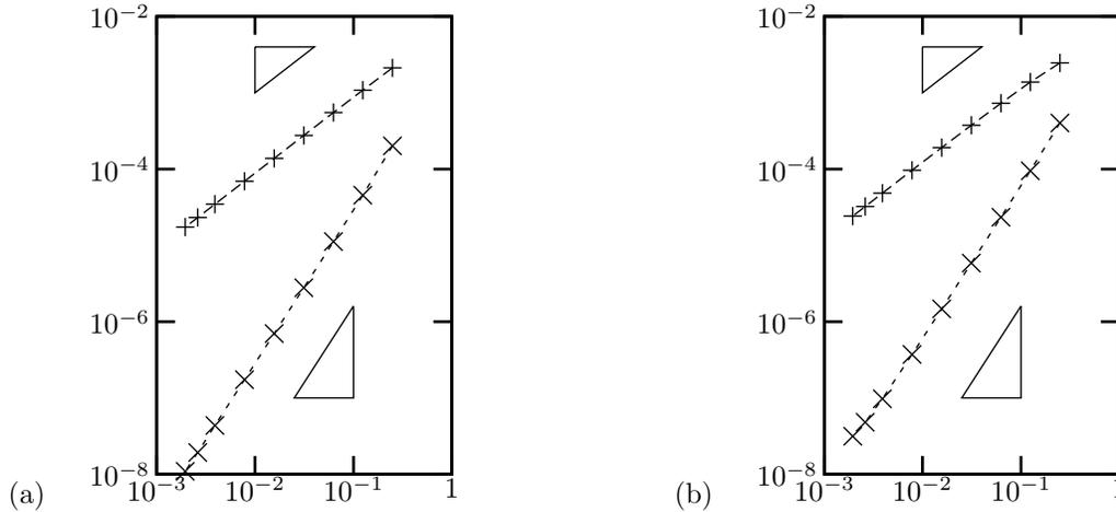
Figure 1. Error  $\max_n \|\mathbf{u}_h^n - \mathbf{u}(\cdot, t_n)\|_0$  versus  $\Delta t$  for (a), problem (11) and (b), problem (12).  $-\text{+}-$ , algorithm (3), and  $-\text{x}-$ , algorithm (10). The triangles have a ratio of 1 and 2, respectively.
