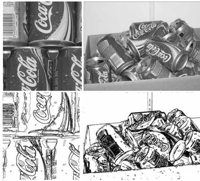
Figure 23: “Coca-Cola” experiment: original images and maximal meaningful level lines. Top: images, bottom: meaningful level lines [5].
