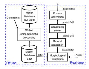
Figure 2: Overview of the motion adaptation process.
