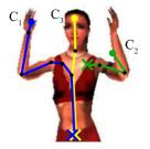
Figure 7: Constraints are associated to a subset of the complete kinematic chain. The three different constraints are represented with big dots. The lines are their kinematic chains and their root are represented with the big crosses.
