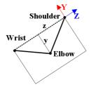
**Figure 4:** Specification of the half-plane represented by the frame (X, Y, Z) which contains the elbow. The local coordinates (y, z) of the elbow are computed analytically.
