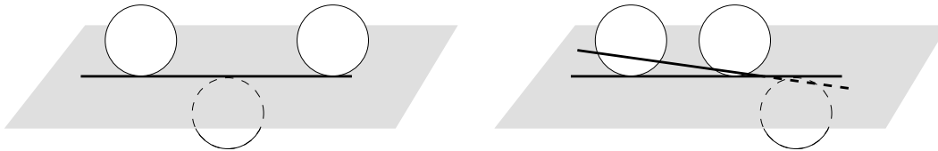
Figure 4. Three spheres with a common tangent plane.
