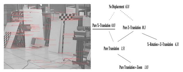
Fig. 9. A partial view of the model hierarchy for a specific displacement estimation. See text for details. The displacement was a pure translation in the X-direction.
