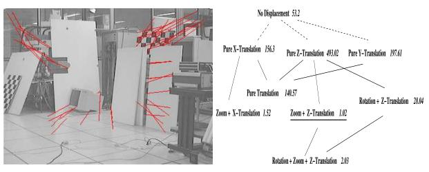
Fig. 10. A partial view of the model hierarchy for a specific displacement estimation. See text for details. The displacement was a zoom of the camera.
