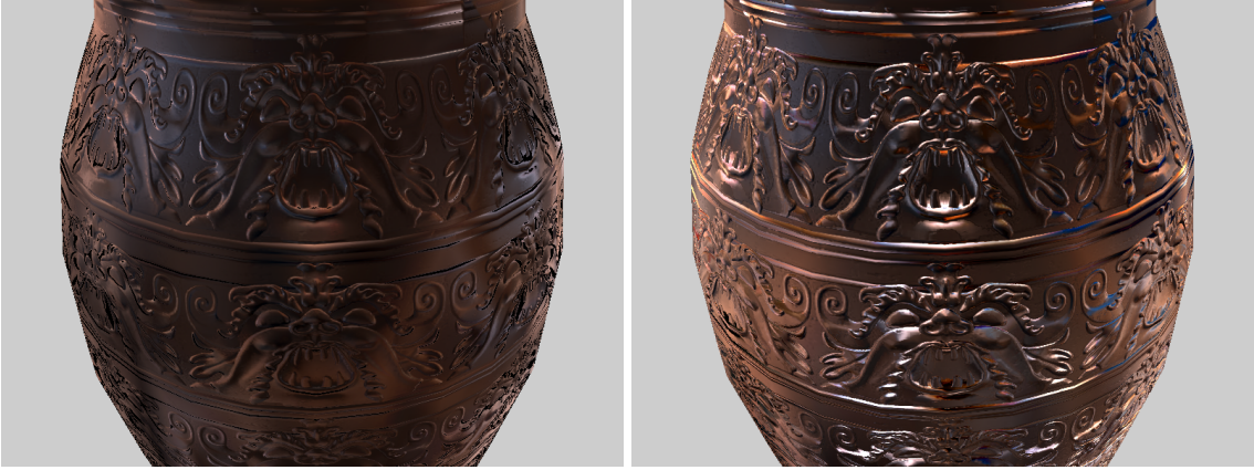
Figure 4: Detail of a normal mapped vase rendered with our SH rotation (right) and with the simplified normal mapping (left). Normal mapping with our SH rotation is more successful at conveying the shape approximated by the normal map. The vase is illuminated by the St Peter’s Basilica environment map; the BRDF comes from a measurement of a brushed metal [Wes].
