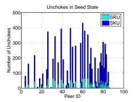
Fig. 7. Number of time each peer is unchoked when the local peer is in the seed state.
