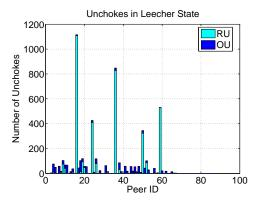
Fig. 3. Number of time each peer is unchoked when the local peer is in the leecher state.
