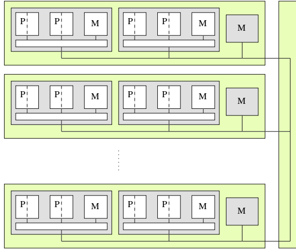
(a) A NUMA of HyperThreaded multicores.
