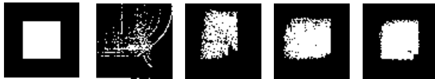
Figure 11: Genetic Programming for Mixed IFS on a 64x64 target. From left to right : target and best images of generations 10, 100, 300 and 1,500. Population size 30 individuals.
