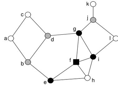
Fig. 1. Application of MPR algorithm: MPR sets are  $\{g, e, i\}$  for node  $f$ ,  $\{d, j\}$  for  $g$  and  $\{b\}$  for  $e$ .
