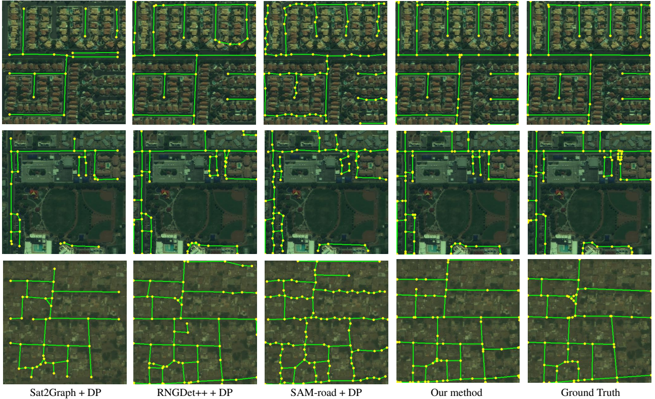
Figure 5. Qualitative results on SpaceNet. Simplifying the results of Sat2Graph, RNGDet++, and, to a lesser extent, SAM-road by a Douglas-Peucker (DP) algorithm produces low-complexity graphs but exhibits geometric and topological inaccuracies. Our algorithm directly returns concise graphs that are similar to the low-complexity ground truth.
