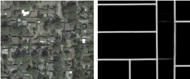
Figure 3. Centerline extraction. The centerlines (right, thin red lines on white pixels) are extracted as the one-pixel-thickness skeleton from the probability map. Note that centerlines are often wavy at some locations: this pixel-level noise is typically absorbed by the line-segment detector.
