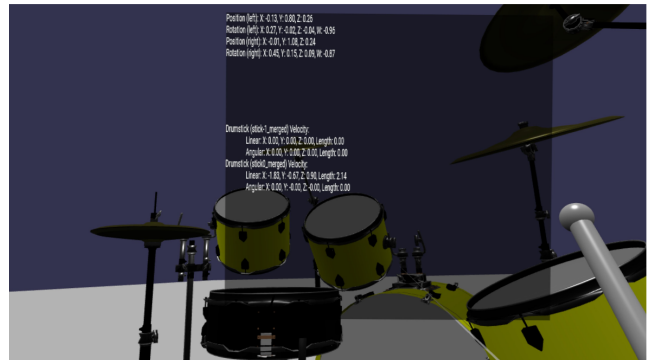
Figure 8: A drum kit / MIDI note generator WAM with a dedicated 3D GUI loaded by custom code for animating its elements depending on the velocity (3D model file created with Blender). Here with a debug panel showing the measured velocity at impact and the generated MIDI events/notes.
