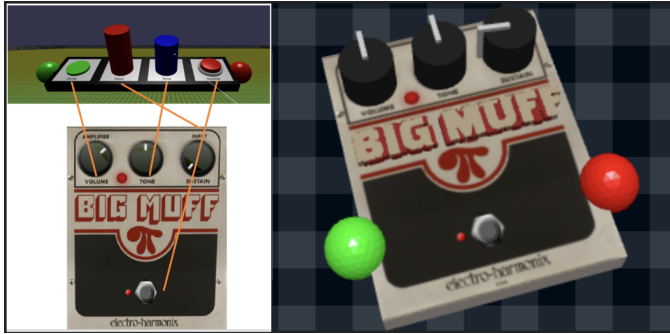
Fig. 2. Auto-generated 3D GUI compared to a custom 3D GUI made with the new 3D editor.
