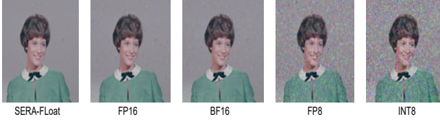
Fig. 7: Image sharpening evaluation results for a female portrait under the F2E2 fault model, involving 2% 1-bit flips and a 0.04% 2-bit flips, across various data formats.
