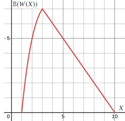
(b) Graph of \mathbb{E}(W(X)) . The maximum is X_{opt} = b with a = 1, b = 3, R = 10, \lambda = \frac{1}{2} .
