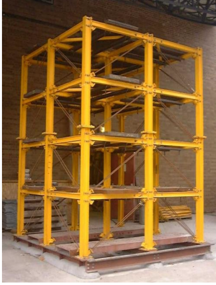
(a) Steel-frame quarter-scale model structure [72]
