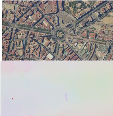
Figure 3. Flow computed with RAFT on the Placa-Tarraco sequence (images of size 1800 \times 950 ). Top: sample image of the sequence. Bottom: estimated flow. Flows are represented using the usual HSV color code (see the supplementary material) with a post-processing for a better visibility. The flow on the vehicles moving along several streets or in the roundabout is mostly absent.
