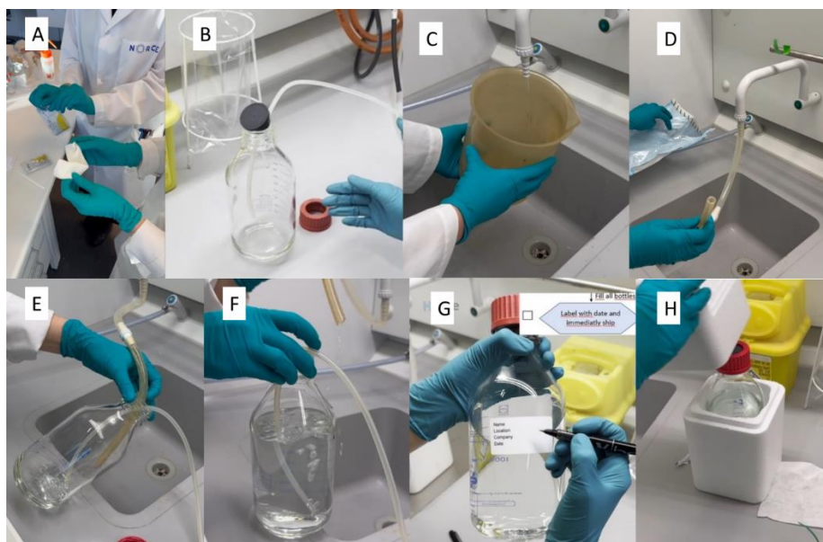
Figure 6: Sampling procedure proposed by our project to obtain anoxic samples for microbiological analysis at the wellhead: (A) Wear gloves and sterilize them before you start. (B) Flush the provided glass bottle with the nitrogen. (C) Flush the pipes properly before sampling. (D) Connect the tubing to the tap. (E) Sample the water while continuously flushing the bottle with nitrogen. (F) Fill the bottle to 2/3 volume and continue flushing with nitrogen. (G) Close the bottle and write the label. (H) Pack the bottle into a Styrofoam box.
