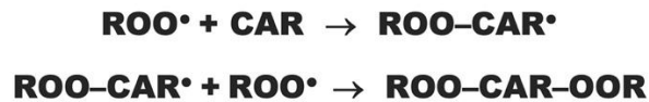
Figure 4.12. A) topological formula of a \beta -carotene molecule. B) simplified reaction between \beta -carotene and free radicals (Britton, 1995)
