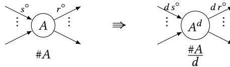
Fig. 12. Firing reduction of actor A by divisor d .
