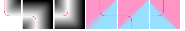
Fig. 6. Left : Transition function b_r in R_o^2 for smooth union, intersection, and difference. The blends are properly closed on the edges of the domain due to the base operators’ bounded property. Right : Color mixing ratio between operands emphasizes the localized influence of each operand in space.
