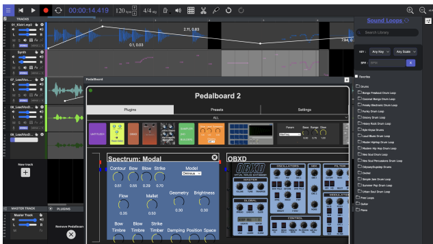
Figure 1: WAM Studio typical view, showing audio and MIDI tracks with some parameter automation curves and the plugin chain associated with the selected track.
