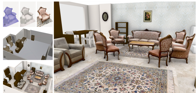
Figure 1: “Cultural Windows” workflow for immersive global interiors: (a) 3D scanning unique design elements, (b) Ensuring privacy with generic, non-photorealistic models, (c) Incorporating 3D models with original textures, and (d) Finalizing the scene for VR.
