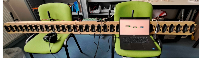
Figure 12. The WFS diffusion system [27] connected to the FPGA Zybo board.
