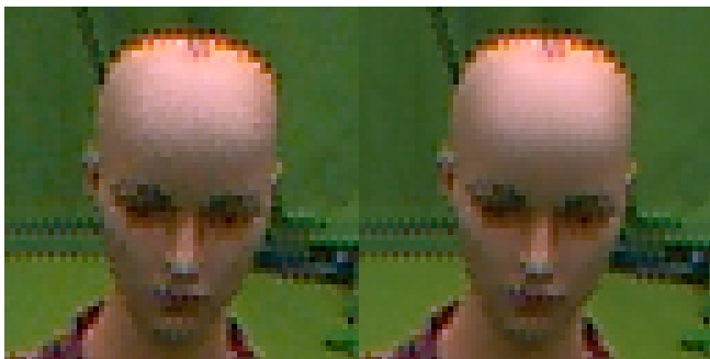
Fig. 4. The camera sensors display some level of noise (left) that can be alleviated by temporal averaging (right) but color fringing and staircase artifacts remain due to the Bayer filter.
