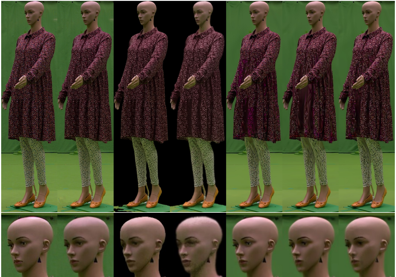
Fig. 7. Qualitative rendering comparisons on the female "cos" scene. Left to right: input image, Ours, Voxurf, Neus2, 3DGS, 2DGS, GOF. The gaussian splatting methods achieve a good image quality overall but tend to fit highly anisotropic gaussians in textured regions, which impacts the extracted geometry in 2DGS and GOF's cases. Neus2 suffers from noise while Voxurf creates sharp boundaries at depth discontinuities. Our method reconstructs both smooth edges that accurately blend with the background image and detailed textured patterns.
