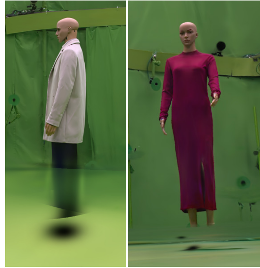
Fig. 1. Convergence failures for gaussian opacity fields (left) due to gaussians near the cameras occluding the scene, and for 2D gaussian splatting (right) due to gaussians above the ground occluding the feet.
