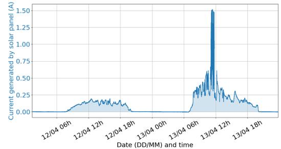
Fig. 2: Photovoltaic energy production of east-oriented solar panel
