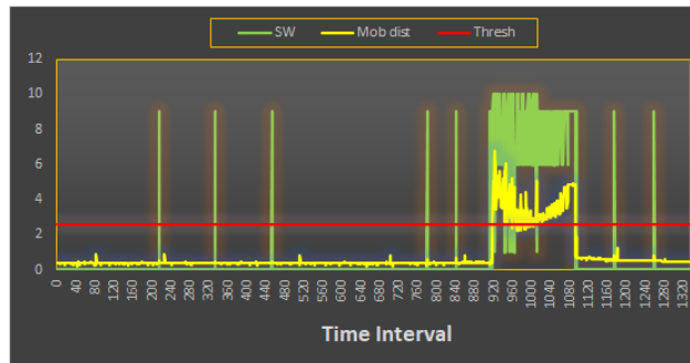
Fig. 12. Comparison Plot of our Sliding Window technique vs Mahalanobis distance vs Threshold
