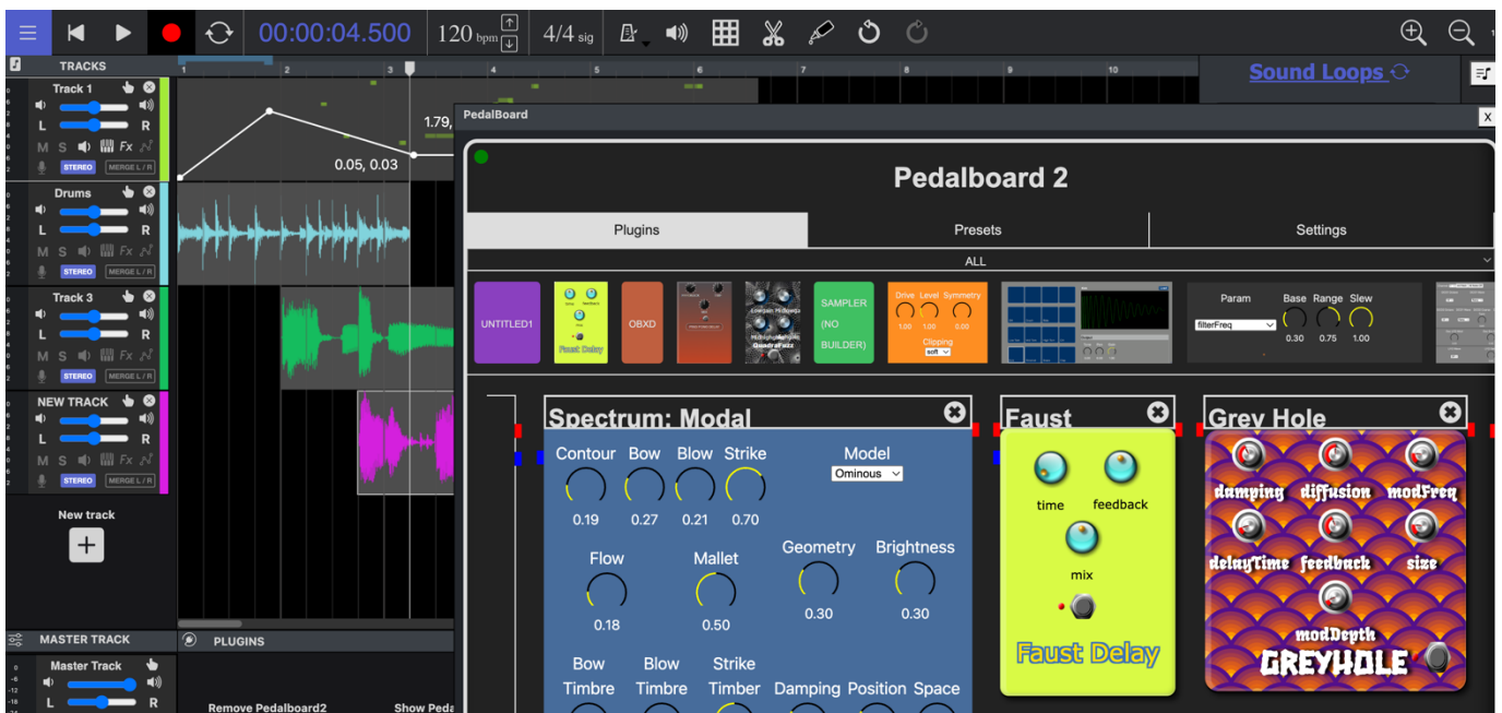
Figure 12: WAM-Studio typical project with MIDI and audio tracks, virtual instruments and effects associated to a track.
