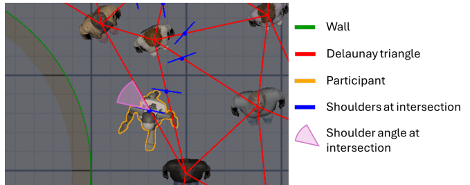
Fig. 6: Shoulder orientation calculation. We first calculate the Delaunay Triangulation, of which the virtual agents are the vertices. Then, when participants cross any edge of any Delaunay triangle, we measure the angle \in [0, 90]^\circ formed by their shoulder segment (left to right shoulder, computed from motion data) and the crossed edge.
