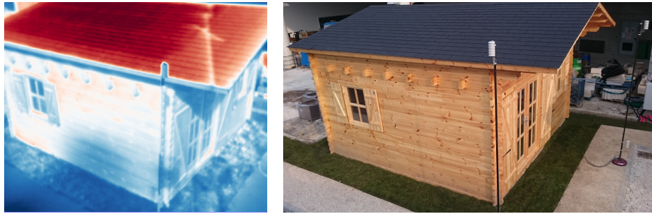
(a) Image of the wooden chalet in the infrared spectrum (b) Image of the wooden in the visible spectrum
