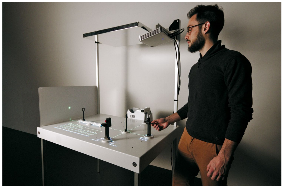
Fig. 1 Photo of the HOBIT, which consists of a realistic optical table equipped with repositionable fake optomechanical components working as a real-time and self-adaptive setup. The calculated optical pattern is displayed on a vertical visualization screen, while pedagogical supports are projected on both the projection screen and the table itself, co-located with the related physical components
