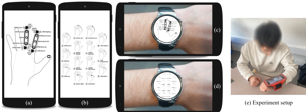
Fig. 14. Experiment conditions: (a) the simultaneous representation of microgestures displayed on a smartphone or (b) the baseline displayed on the same smartphone and (c) the simultaneous representation of microgestures displayed on a smartwatch or (d) the baseline displayed on the same smartwatch. The smartwatch was (e) simulated by a smartphone
